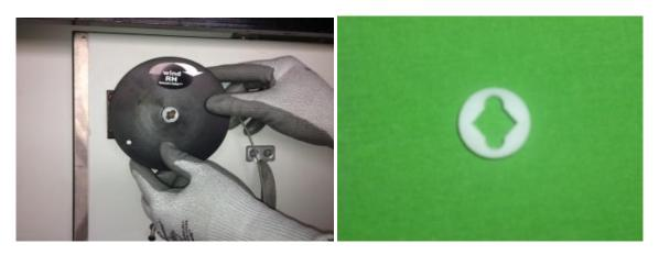
2) Mount spirator RH or LH (marked on unit) to active panel in door closed position. 1/8" shims provided as needed.
