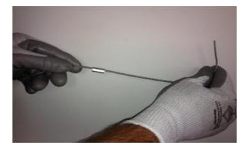
**3)** Determine fastening point, washer or "S" hook may be required at fastening point, unwrap appropriate length of cable to fastening point. Remove loose end of cable from sleeve and wrap around fastening point and feed back through sleeve.
